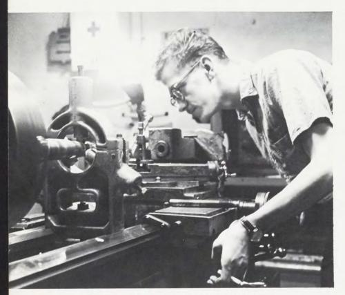
Machine shop lathe operator turns motor shaft for a small bdy
