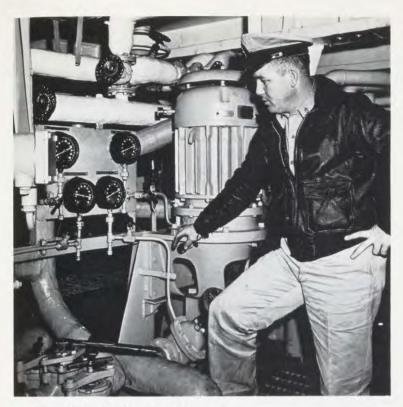
V-4 Chief Checks Pressure Readings On Lube Oil System
