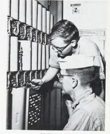
IC Electricians Mates repair ship's telephone system
