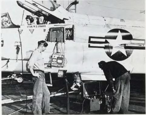
Testing Electrical System on F8U
